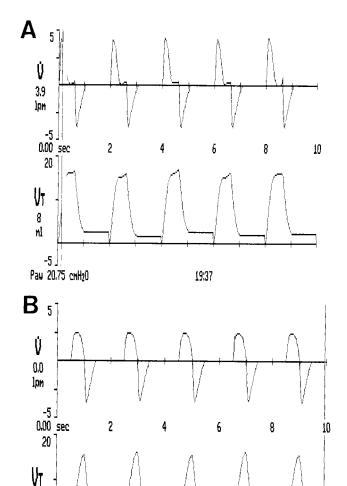
Fig. 5. Cycling mechanisms. A: Time cycling. Note how the flow waveform (top) returns fully to baseline and expiration does not begin until the inspiratory time limit has been reached. This results in a plateau on the volume waveform (bottom). B: Flow cycling. Note how the flow waveform (top) cycles directly from inspiration to expiration prior to reaching a zero-flow state. The resulting volume waveform is peaked.  $\dot{V}=$  flow.  $V_T=$  tidal volume.  $P_{aw}=$  airway pressure.
